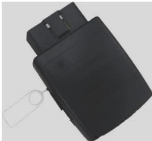
2. Place the micro-SIM card on the tray with the gold-colored contacts facing down and slide the tray back into place.
